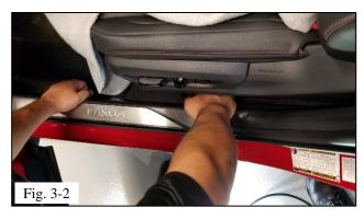
(b) Remove the front driver door sill by disengaging the hooks located at the rear and front of the door sill and pulling up on the door sill. Discard the front driver door sill (Fig. 3-2).
