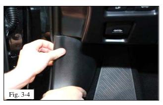
(d) Remove the cowl by pulling rearward and inward to disengage two (2) attachment clips and retain for reassembly (Fig. 3-4).
