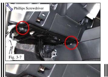
(g) Remove two (2) 8 mm bolts from the IP undercover and retain for reassembly (Fig. 3-7).
