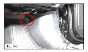
(c) Remove the plastic nut on the cowl and retain for reassembly (Fig. 5-3).
