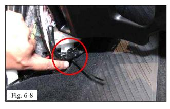
(h) Route the illuminated door sill harness below the junction block in the cowl area and use one (1) zip tie to attach the illuminated door sill harness to the vehicle harness (Fig. 6-8).
