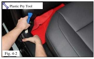
(b) Use a nylon pry tool to disengage hooks located on front of the door sill (Fig. 4-2).
