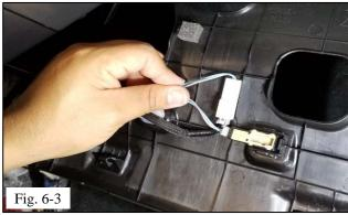
(c) Remove the OE foot lamp connector and replace with illuminated door sill connector. Connect the OE connector to the illuminated door sill connector. Bundle the wire harness and connector (Fig. 6-3).
