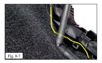
(g) Use one (1) zip tie to attach the illuminated door sill harness to the vehicle harness near the bottom of the junction block. The zip tie lock should be pointed away from the window washer tube (Fig. 8-7).
