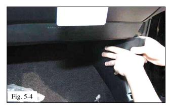
(d) Remove the cowl by pulling rearward and inward to disengage two (2) attachment clips and retain for reassembly (Fig. 5-4).
