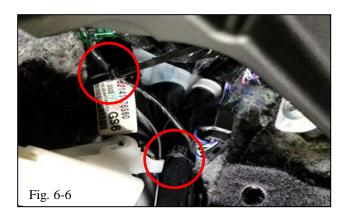
(f) Route the illuminated door sill down towards the cowl area and use two (2) zip ties to attach the illuminated door sill harness to the vehicle harness (Fig. 6-6).
