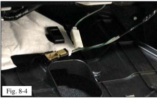
(d) Remove the OE foot lamp connector and replace with illuminated door sill connector. Then connect the OE connector to the illuminated door sill connector (Fig. 8-4).
