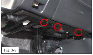
(h) Disengage the three (3) clips holding the IP undercover in place (Fig. 3-8).
