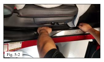
(b) Remove the front passenger door sill by disengaging the hooks located at the rear and front of the door sill and pulling up on the door sill. Discard the front passenger door sill (Fig. 5-2).
