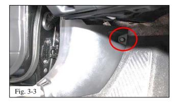
(c) Remove the plastic nut on the cowl and retain for reassembly (Fig. 3-3).
